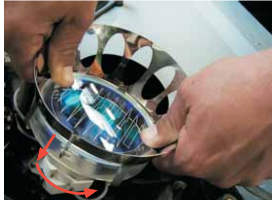
Illustr. 5-6-4: Unscrew the reflector
