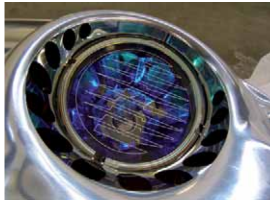
Illustr. 5-6-8: Reflector correctly positioned under the chrome cover
