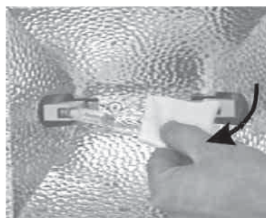
Illustr. 5-13 Pulling the burner out towards the front
