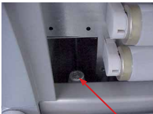
Illustr. 5-18 Left tension screw
