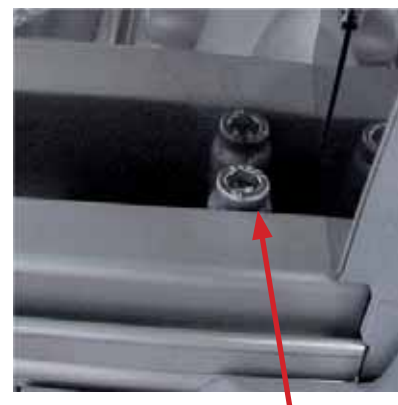
Illustr. 5-19 Right tension screw
