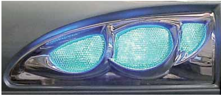
Illustr. 5-15 LEDs in the canopy of KBL 6800, on the right
